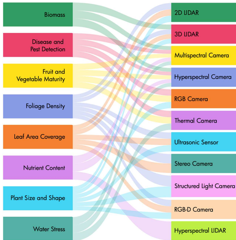
Figure 2.2: RS instruments and their uses (Botta et al., 2022)
