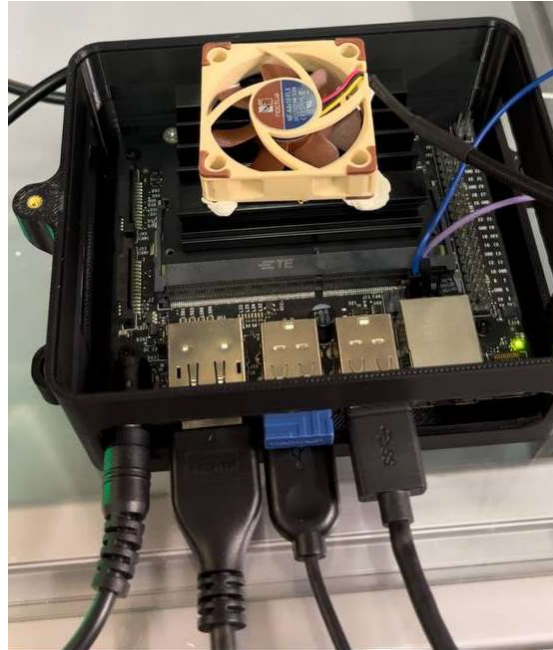
Figure 2.6: NVIDIA Jetson Nano with fan and (open) custom case
