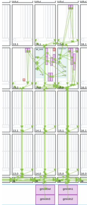
Figure 6.3. Bilinear kernel graph after compilation - array view
