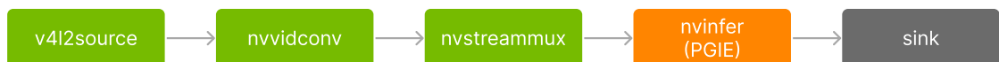
Figure 4.2: Simplified Video Source Pipeline, a minimal pipeline using a camera video feed
