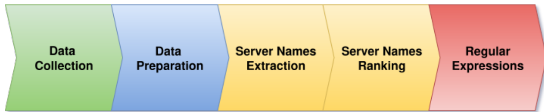
Figure 4.1: Pipeline and operational steps for discovering live streaming server names associated to a content provider
