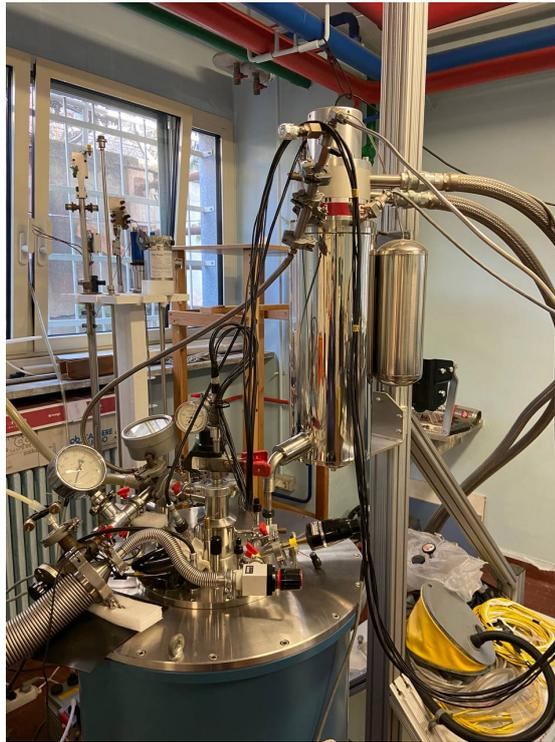
**Figure 6.9:** *The figure shows the LaTEST 1 cryocooler, integrated with the recondenser. Here, the descendant was inserted for point-contact measurements.*
