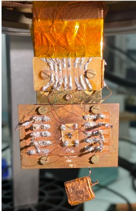
**Figure 6.7:** *The figure shows the vertical setup, ready to be closed by the metal shield, which prevents thermal fluctuations during the measurement. At the bottom, we can see the thermometer, which is typically linked through G.E. Varnish behind the sample's copper support.*
