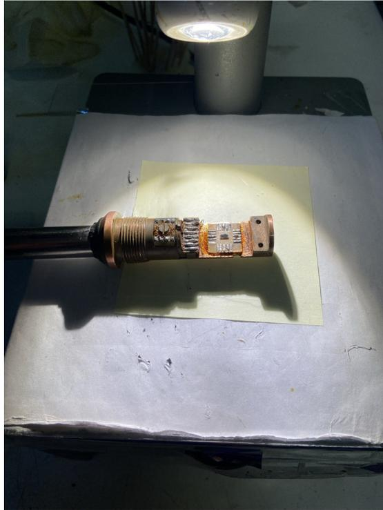
**Figure 6.5:** *Sample chamber of the cryogenic insert used in the Oxford top-loading wet cryostat. Here, the sample was prepared for soft-point contact measurement, so the pool was not necessary.*
