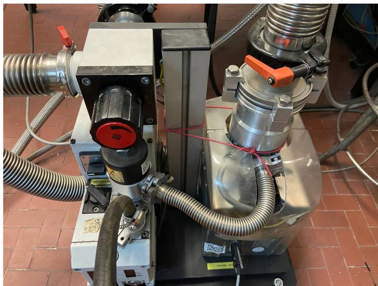
**Figure 6.10:** *The image shows, on the left, the booster pump, responsible for maintaining low vacuum conditions, and on the right, the turbo pump, which is tasked with achieving high vacuum.*
