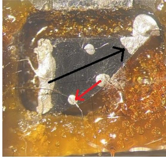
**Figure 6.1:** *Example of  $Fe(Se,Te)$  mounting. We can see the G.E. Varnish in the background, on top the sample with the Ag-spots. The black arrow define the flow of the drain-source current ( $I_{DS}$ ), while the red arrow indicates the voltage drop between two electrodes*
