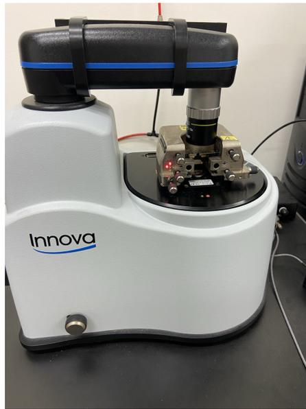
**Figure 7.3:** *Innova Bruker atomic force microscope.*
