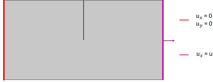
Figure 5.1: Schematic representation of the single-edge notched plate problem.
