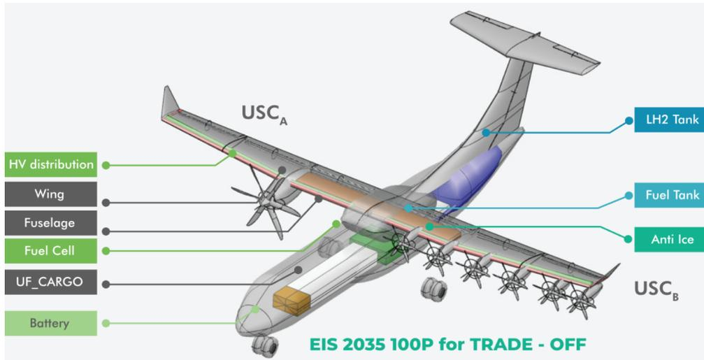
Figure 1.4: USCs concept trade-off and possible concept configuration [8]
