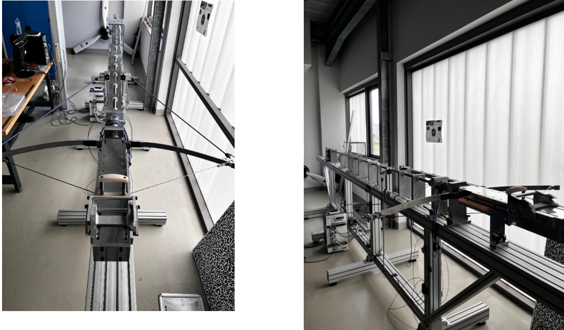
Figure 6.33: Split Hopkinson pressure bar setup at ISAE-Supaero
