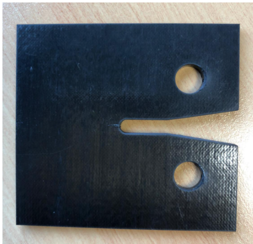
Figure 5.9: CC coupon after test
