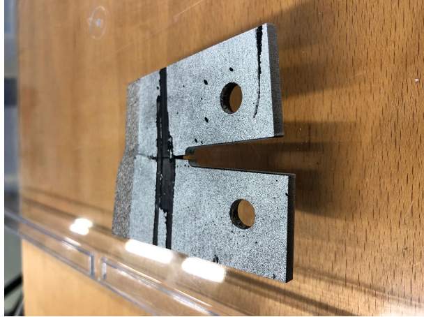
Figure 4.13: CT Coupon after test
