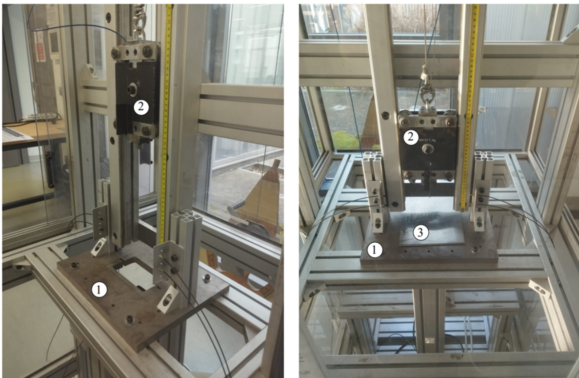
Figure 88: Experimental machine for impact tests: "1" indicates the steel base plate with the window to observe the posterior deflections of the impacted plate, "2" indicates the loading system (i.e. the impactor with an accelerometer connected to the impact mass). The image on the right shows the placement of the aluminum plate ("3") above the window.
