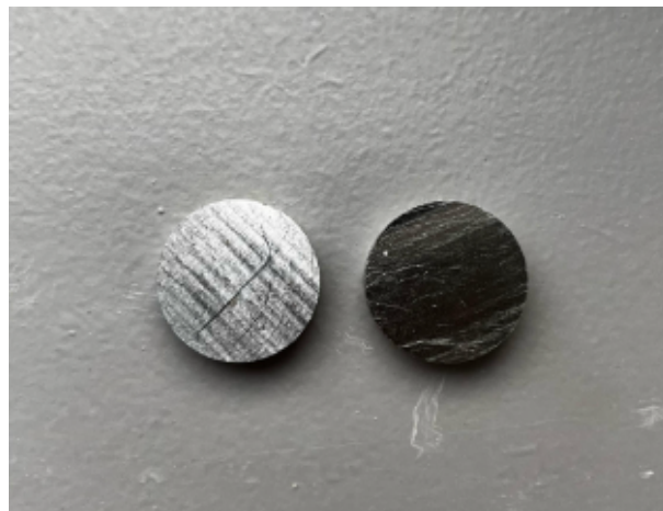
Figure 47: Tungsten carbide spacers used in high velocity Hopkinson bar tests.
