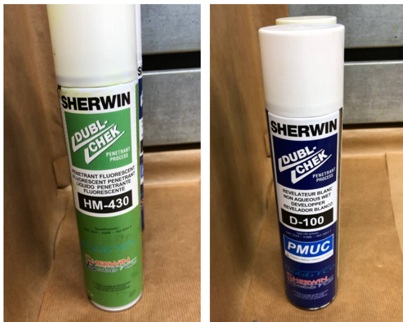
Figure 30: Penetrant liquid (left) and developer (right).
