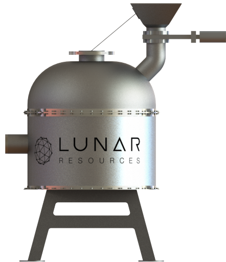
Figure 4.15: Rendering of a molten resource extractor under development by Lunar Resources
