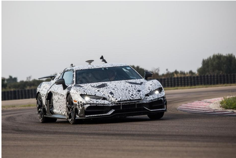
Figure 15: A camouflaged master vehicle during track testing, some sensors are visible on the extern. .21
