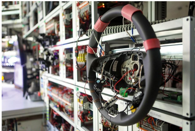
Figure 9: Within the modules, ECUs are wired to special probes. .14
