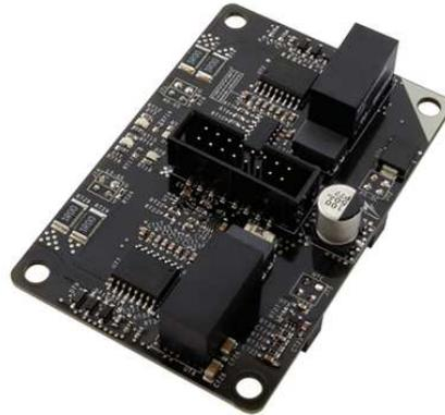
Figura 3.18: Schede Gate Driver del kit Wolfspeed.
