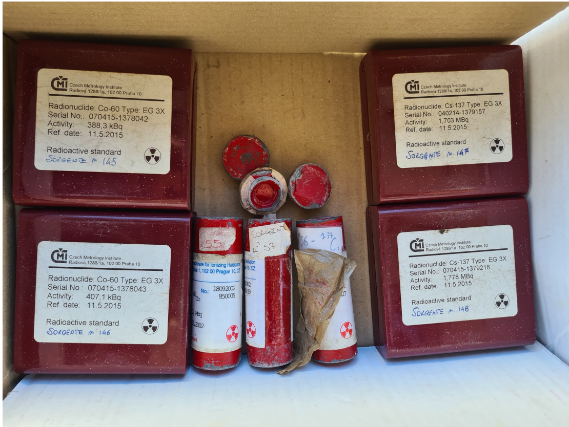
Figure 5.5: Box containing the protective cases for the sources used in the study. Two ^{137}\text{Cs} sources, still inside their sealed containers, were left on the window ledge. Their larger size prevented their use in the experiment, but their proximity to the setup caused an unintended contribution to the radiation measurements.
