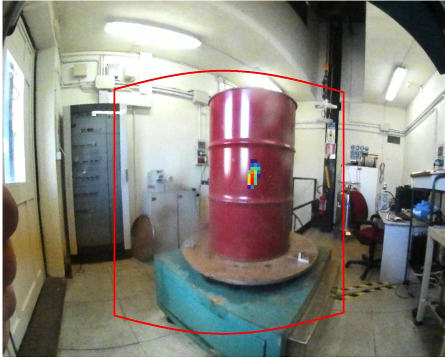
Figure 3.4: Example of CAI reconstruction of a ^{241}\text{Am} source in a waste container using the GammAware system.
