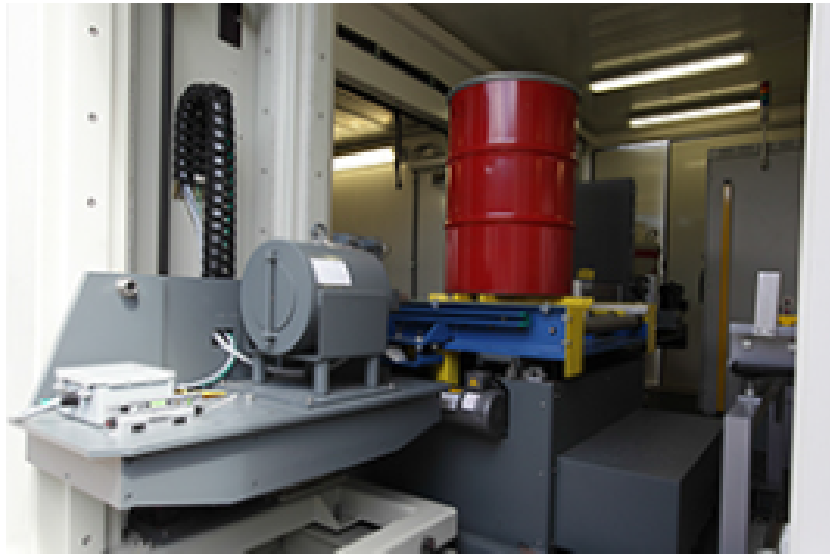
Figure 3.7: The TGS system owned by Nucleco consists of an HPGe detector, a lifting platform for the drum, a roller conveyor for drum transport, and a rotating platform.
