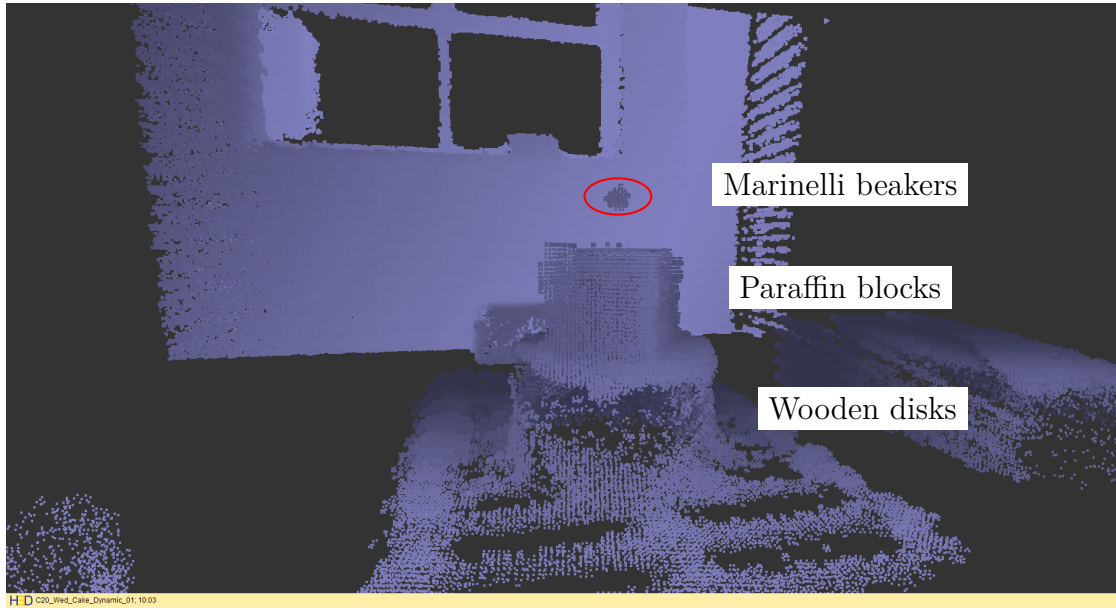
Figure 4.4: 3D point cloud generated by the GammAware device using LIDAR technology. The image has been extracted from H3D Visualizer 3D and has not been edited, except for the removal of part of the surrounding point cloud, including the floor, to improve clarity in visualising the WC and its components. The Marinelli beaker, highlighted with a red circle, appears poorly reconstructed due to the limitations of LIDAR in capturing transparent or low-reflectivity materials.
