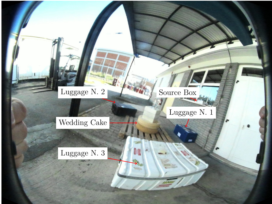
Figure 4.7: Optical image captured by the H420 detector showing the measurement scene. The luggage pieces, the Wedding Cake, and the sources box left on the window ledge are indicated with arrows and labels.
