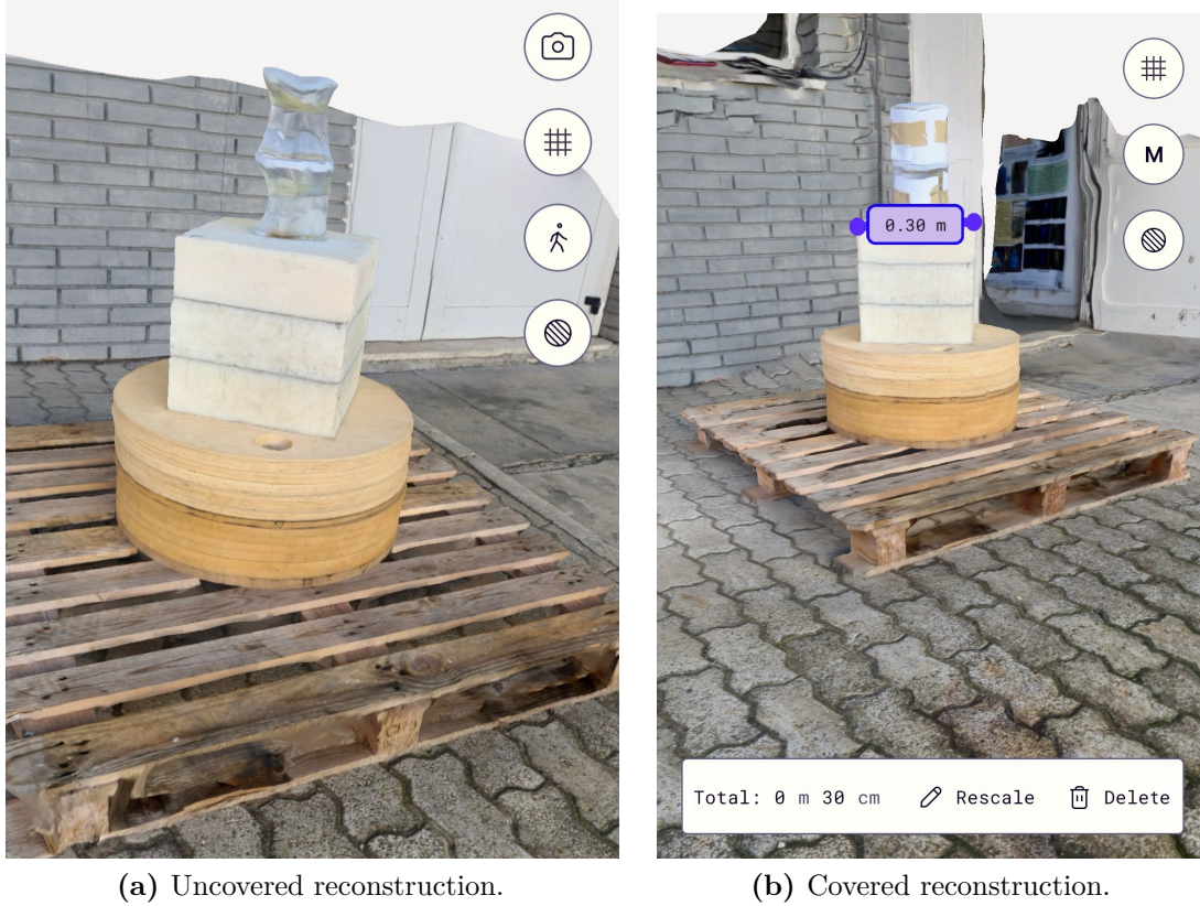
Figure 4.5: Screenshots from the Polycam photogrammetry software [33], captured using a smartphone. (a) Reconstruction of the Marinelli beaker in its uncovered state, showing the original transparency. (b) Reconstruction of the Marinelli beaker covered in paper, performed to enhance the software’s ability to manage transparency. Both images are part of the 3D scene reconstruction.
