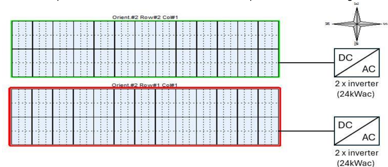
Figure 28: PV modules layout
