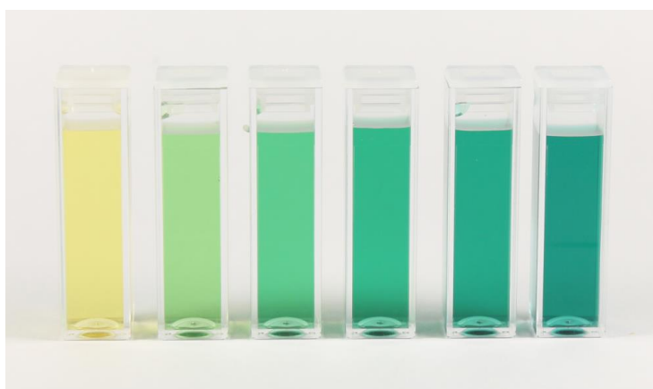
Figure 30: effect of ammonia concentration on the dye [58]
