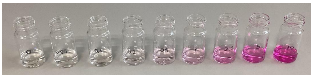
Figure 31: effect of nitrite concentration on the dye
