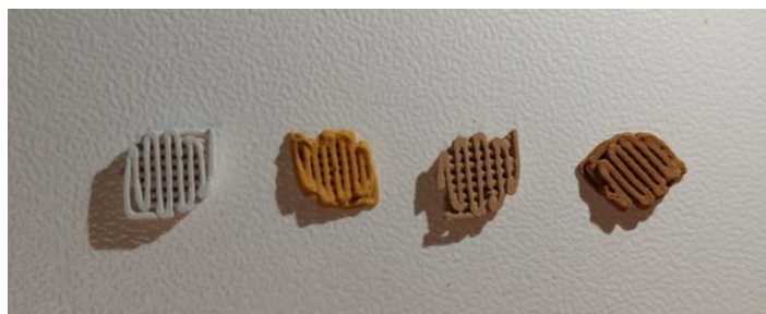
Figure 38. Photograph of the produced scaffolds. From left to right: 100:0 wt%, 95:5 wt% wet, 95:5 wt% dry, 90:10 wt% dry.
