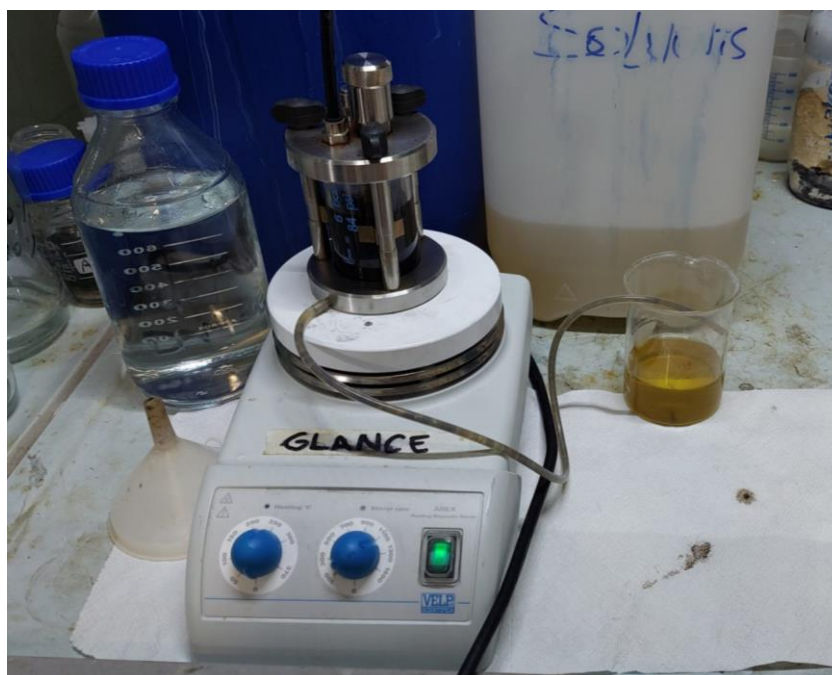
Figure 29. Ultrafiltration of liquid solution of \text{Fe}_3\text{O}_4 NPs and citric acid.
