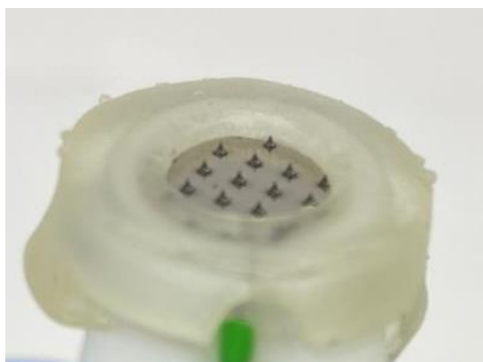
Figure 2 Microneedle-based platinum sensor.
