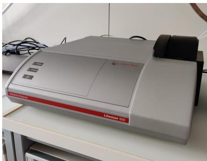
**Figure 31** – Anton Paar Litesizer 500 Particle Analyzer.
