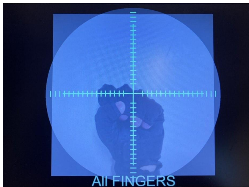
Figure 7: Layout of the experimental setup that was showed on the screen to the subjects during the experiment. Dashes on the cross were at such a distance that the circle, as it tightened, touched each consecutive dash at a frequency equal to the required frequency of movement. ‘All fingers’ refers to the type of movement to perform, always written below the circle.
