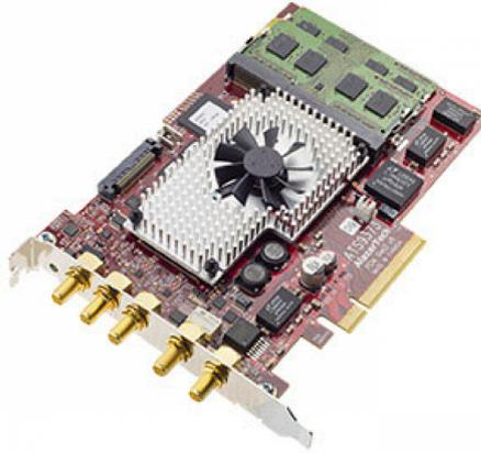
**Figure 2.4:** the ATS9870 DAQ board
