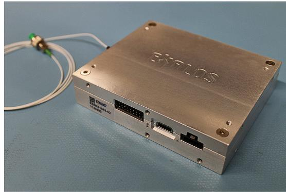
**Figure 2.6:** The 4 SLED laser
