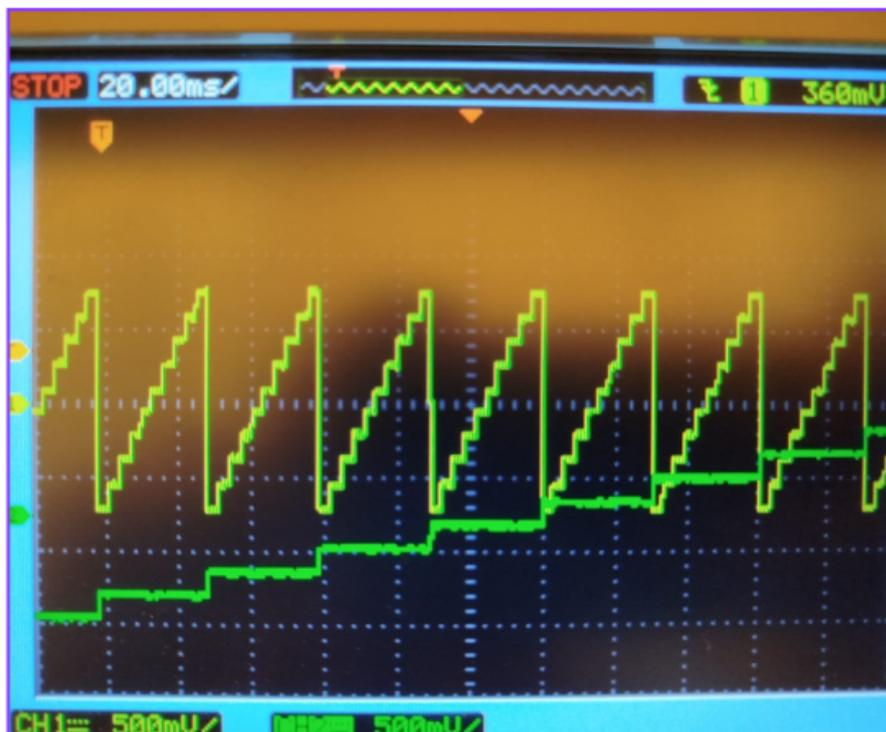
**Figure 4.1:** Signal from the FPGA to the galvos, we can see the fast axis in yellow and the slow one in green
