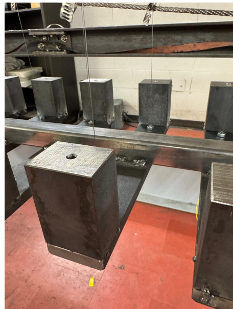
(b) Tensioned hanging system
