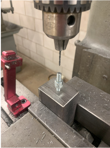
(a) Drilling the hole inside the screw.
