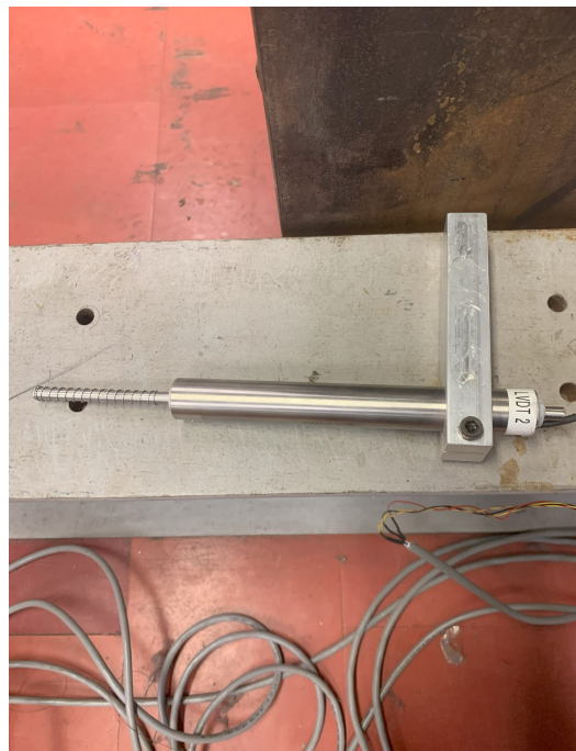
Figure 7.20: LVDT used to calculate displacement in midspan
