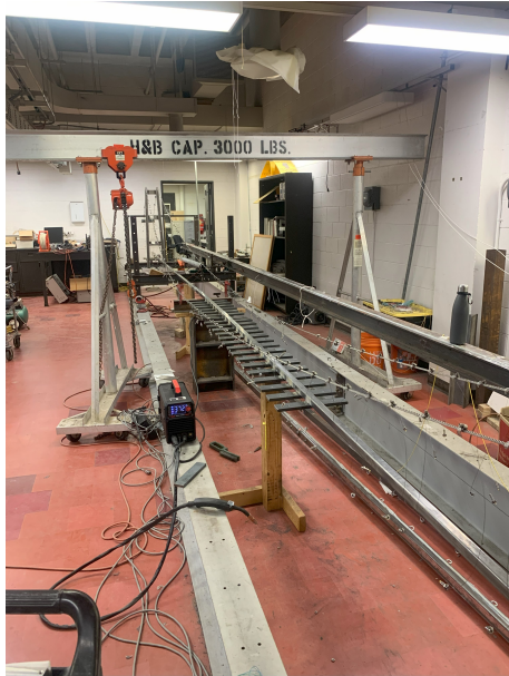
(a) Partial welding of mass plates.
