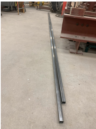
Figure 6.6: Raw bars for the bridge's deck.
