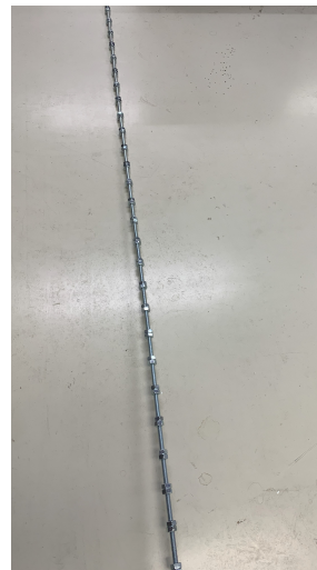
Figure 6.2: Couple of nuts inserted in the bar every 3.81 cm ( 1.5 inches)
