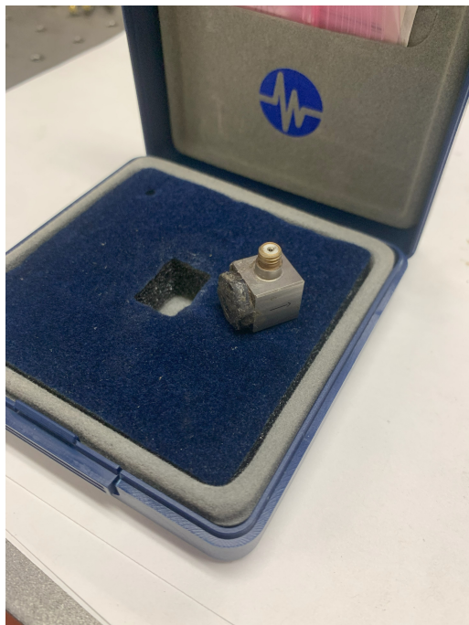
Figure 7.19: Accelerometer used for calculating the dynamic properties of the bridge
