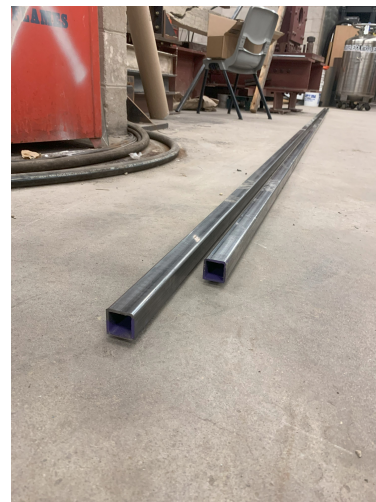
Figure 6.7: Cross-section of the bridge's deck bars HSS 1\frac{1}{4} \times 1\frac{1}{4} \times \frac{1}{8} .
