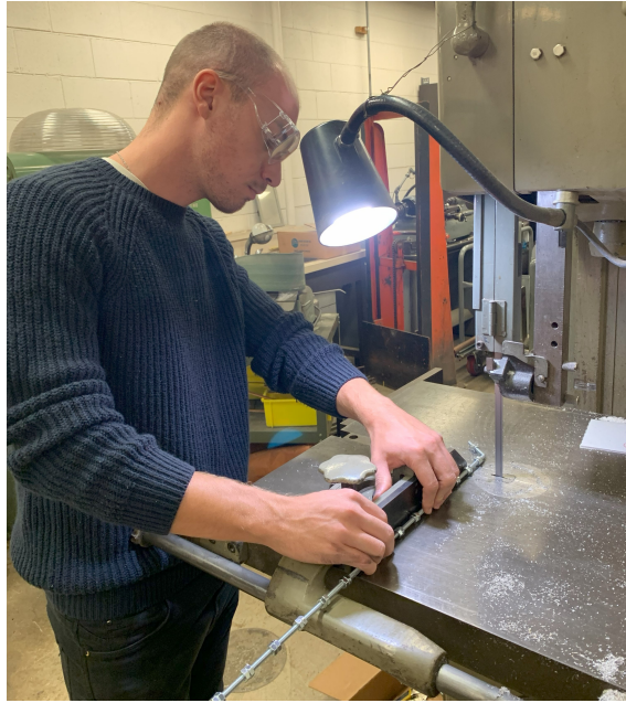
Figure 6.3: Band saw used for cutting the bars in single pieces
