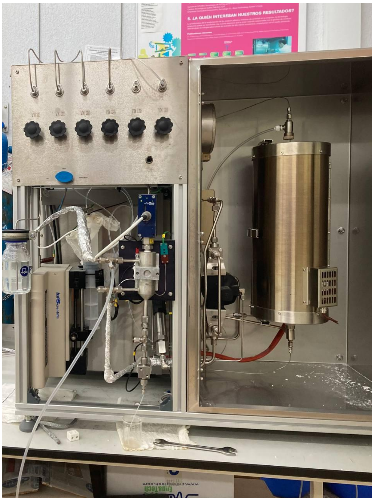
Figure 9.- Photograph of the fixed-bed reactor used in this study, located at the Department of Chemical Engineering of UPV/EHU.
