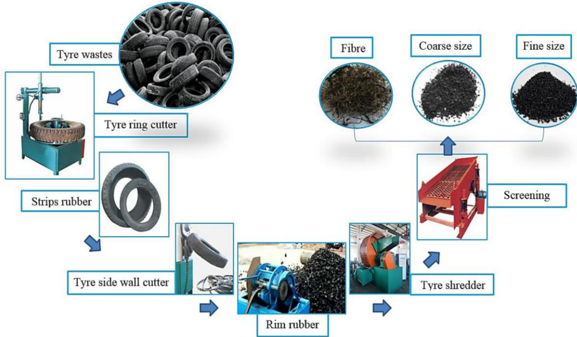
Figure 2-2. Process of shredding of waste tyres. Image from Mhaya et al., 2021.
