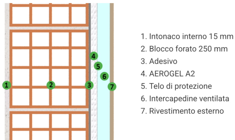
Figure 5 - Stratigraphy of ventilated facades, section. source[5]
