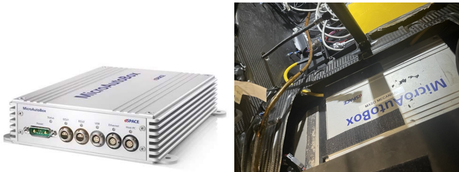
Figure 30: dSpace MicroAutobox II installation
