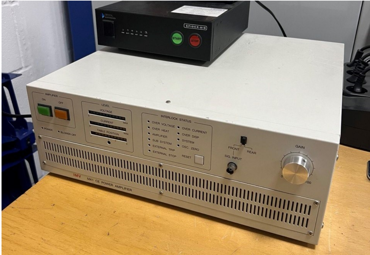
Figure 4.6: Power Amplifier and Vibration Controller
