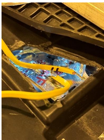
Figure 3.8 Thermocouples T9 and T11 on the LED heatsink
