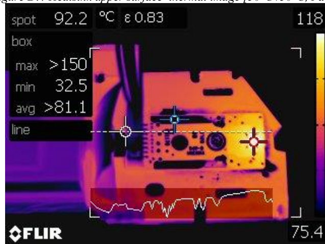
Figure D.4 Heatsink upper surface thermal image [50°C /50°C, Fan Off]
