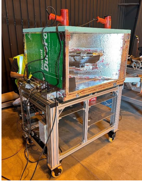
Figure 3.2 Thermal chamber on the fixture, equipped with two heat guns and testing headlamp.
