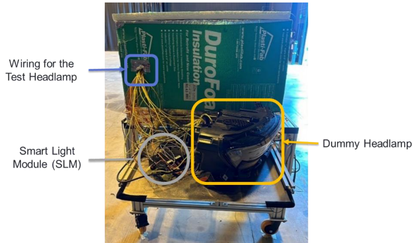
Figure 3.4 Wiring connection and dummy headlamp
