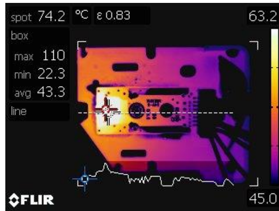
Figure D.2 Heatsink lower surface thermal image [room temperature]
