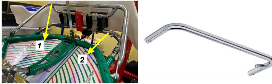
FIGURE 4.73: FRONT BUMPER SYSTEM (1: UPPER BUMPER, 2: LOWER BUMPER) ON THE LEFT, ISOMETRIC VIEW OF THE FRONT LOWER BUMPER ON THE RIGHT.
