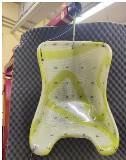
FIGURE 5.22: HANGED GREYHOUND WITH ACCELEROMETERS INSTALLED.
