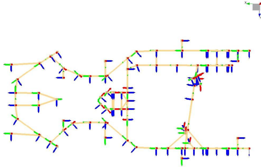
FIGURE 5.16: NODES LOCAL REFERENCE SYSTEM RE-ORIENTED: CHASSIS.
