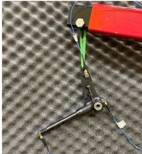
FIGURE 5.38: STUB-AXLE WITH ACCELEROMETERS INSTALLED ON NODES 9, 13, 1.
