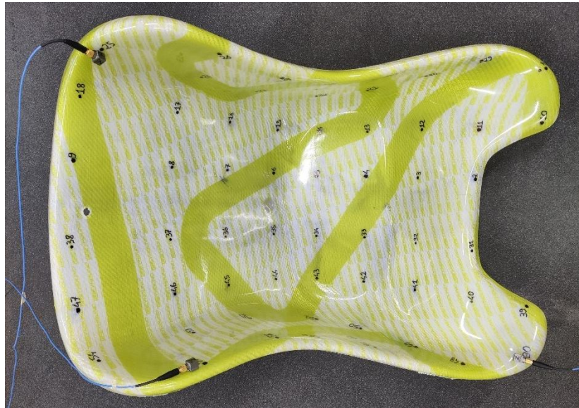
FIGURE 5.7: ACCELEROMETERS POSITIONED ON THE GREYHOUND SEAT.
