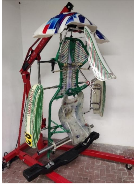
FIGURE 7.16: HANGED FINAL ASSEMBLY WITH ACCELEROMETERS INSTALLED ON NODES 2021, 1001, 1021, 2001.
