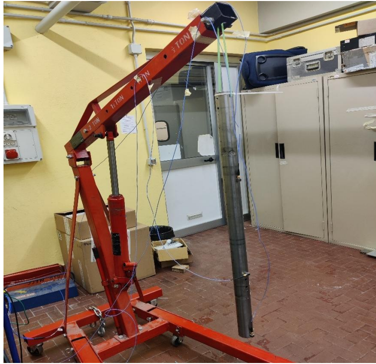
FIGURE 5.4: EXAMPLE OF TEST OBJECT (REAR AXLE IN THIS IMAGE) HANGED BY HYDRAULIC CRANE THROUGH ELASTIC RUBBER BANDS.
