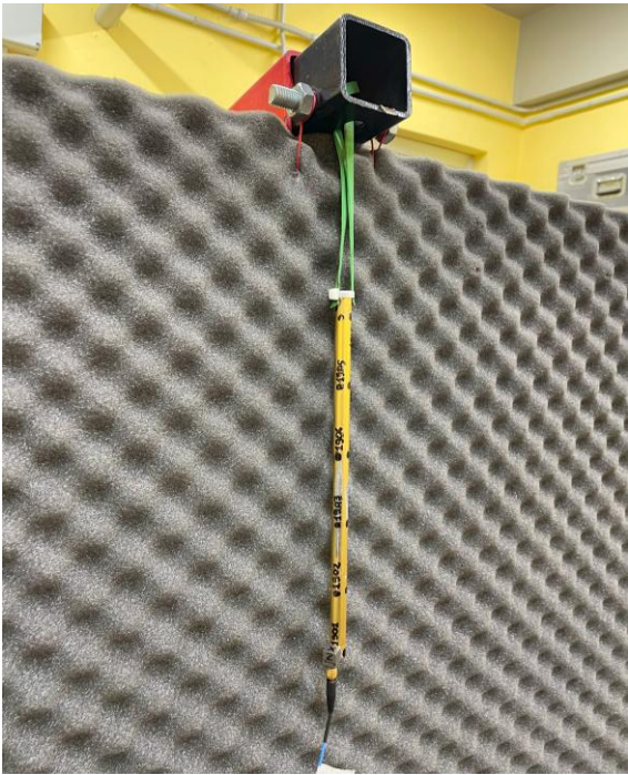
FIGURE 5.35: STEERING TIE-ROD WITH ACCELEROMETERS INSTALLED ON NODE 1.
