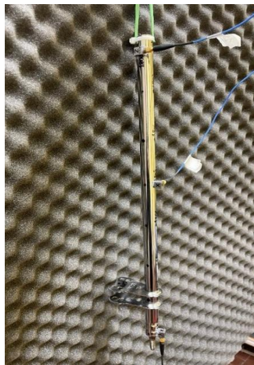
FIGURE 5.32: STEERING COLUMN WITH ACCELEROMETERS INSTALLED ON NODES 10, 1, 5.
