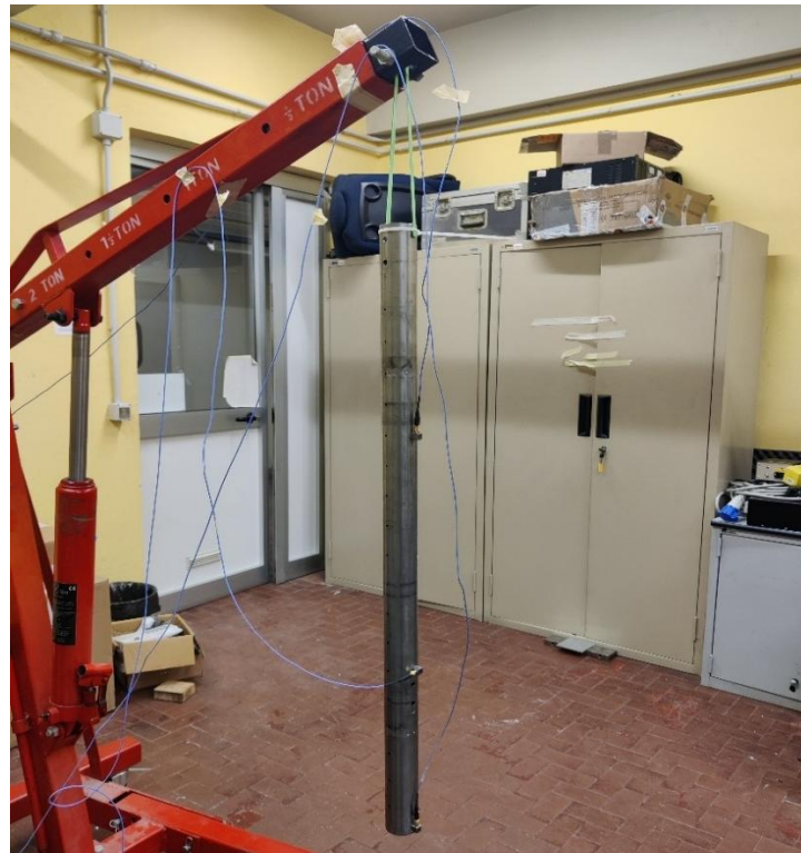
FIGURE 5.25: HANGED FRONT ARB WITH ACCELEROMETERS INSTALLED ON NODES 1, 7, 15.
