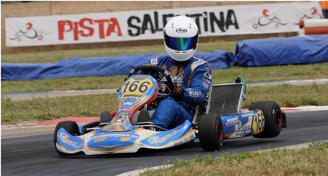
FIGURE 1.4: REAR-LEFT WHEEL RAISED-UP WHILE BENDING A LEFT CORNER.
