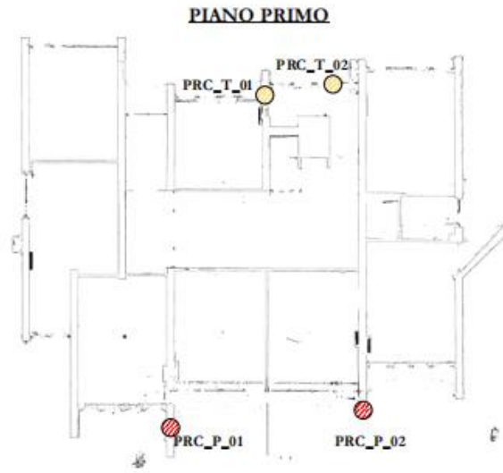
Figure23- Location of material Investigation_First Floor
