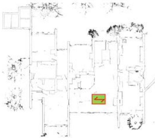
Figure 47-Slab direction _Second structural floor (ORD_S_01)
