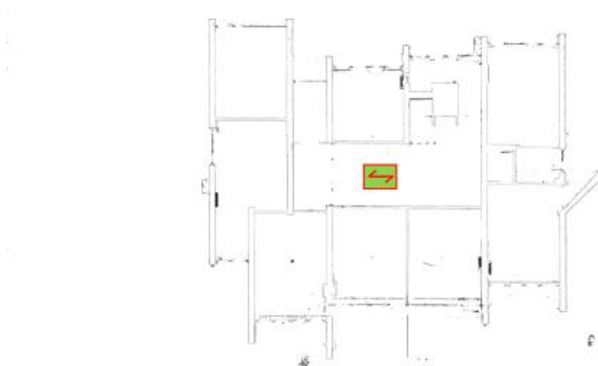
Figure 48-Slab direction_Third structural floor (ORD_S_01)
