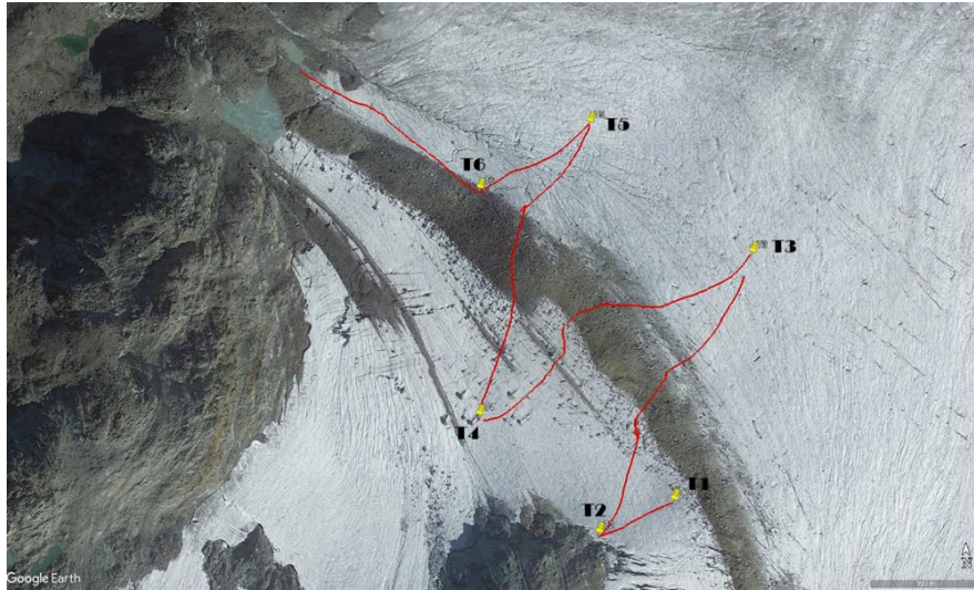
Figure 16 - GPR traces profiles (200 MHz). Symbols T1 to T6 identify the starting point for every line (Godio & Franco, 2024)
