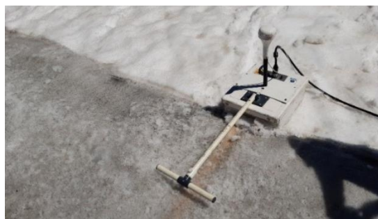
Figure 13 - GPR device (Indren glacier). Photographic material provided by Politecnico di Torino - DIATI
