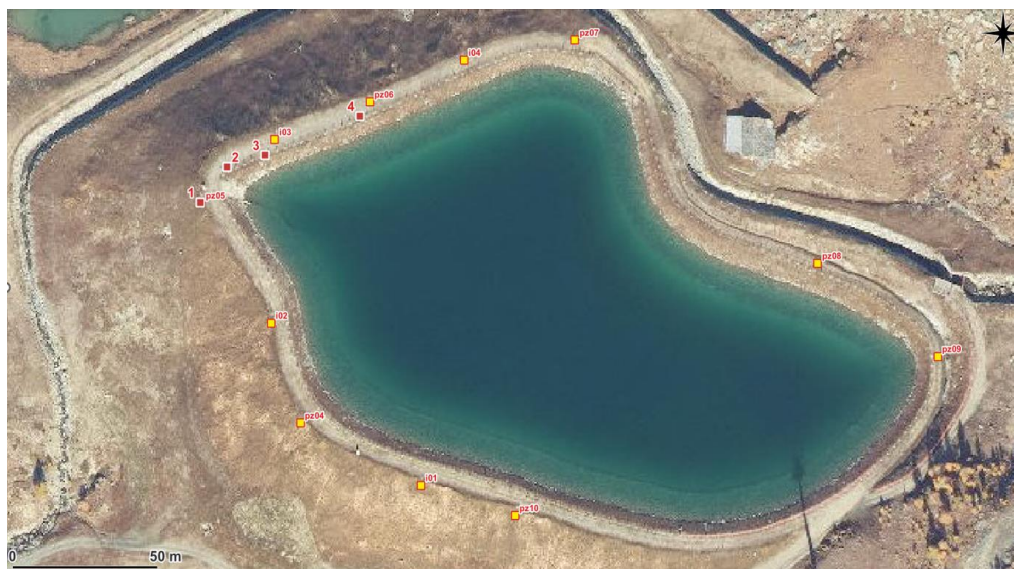
Figure 6 - shows the position of four passive seismic monitoring stations at the Fourcare Embankment; the four red square from 1 to 4 represent the passive seismic monitoring stations while the points (i) show the positions of inclinometers and (pz) are the piezometers.
