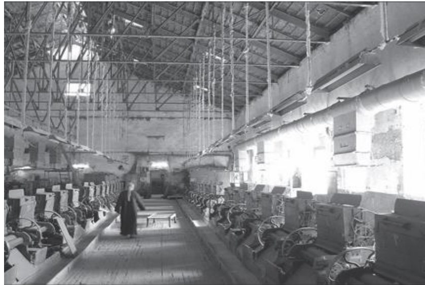
Fig.4.40. The interior of Abdel-Meguid Barakat Ginning Mill (Damanhur) dating back to the early 20th century, featuring the initial timber platform and the operational rolling gins. The mill is still in service today. (Bibliotheca Alexandrina)
