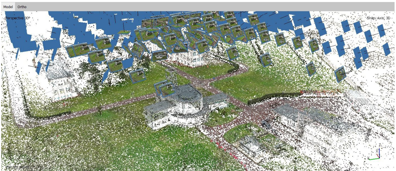
Fig. 32B. Sparse point cloud Aerial Range / 458,181 points.
