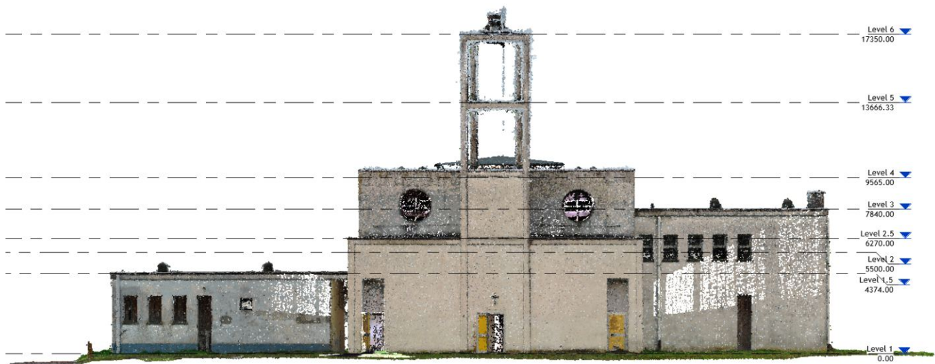
Fig. 29 (below). Levels shown on West Elevation (Not to Scale). Source: By authors – done in Autodesk Revit 2024.
