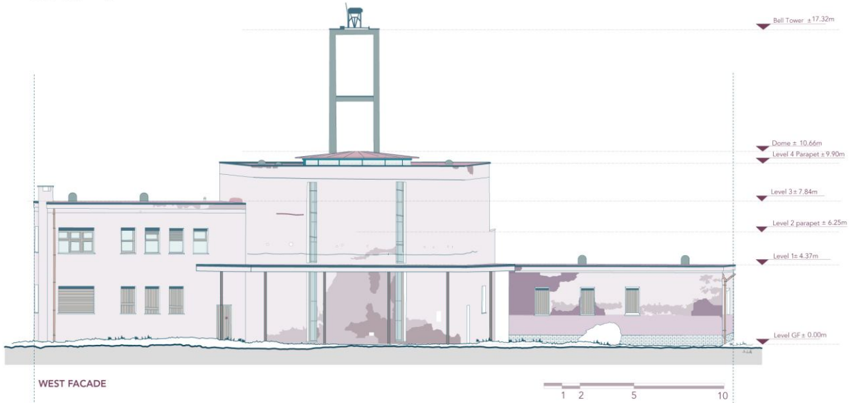
Fig. 21. West Façade Material Mapping in reference to the Orthomosaic. Source: Elaboration by the Authors
