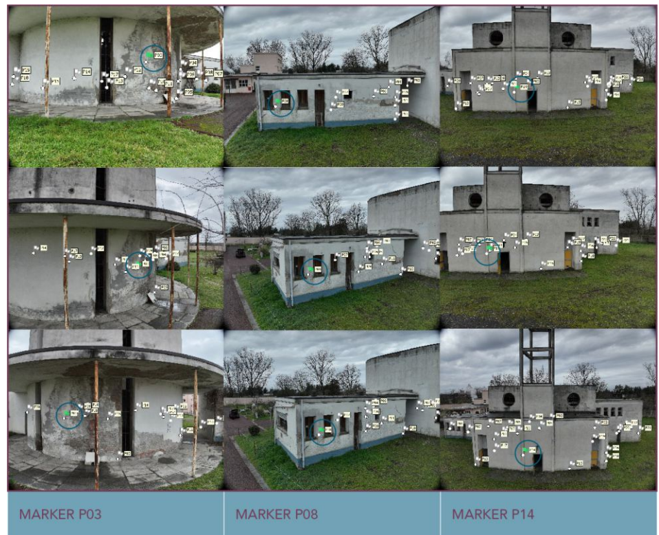
Fig. 36. Placing three markers in three different images in the Aerial close range chunk.
