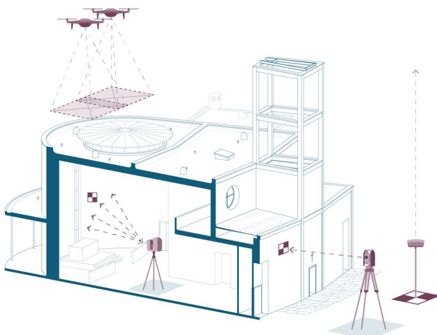
Fig. 1. Tools and methods used in 3D Survey. Source: Elaboration by Authors.
