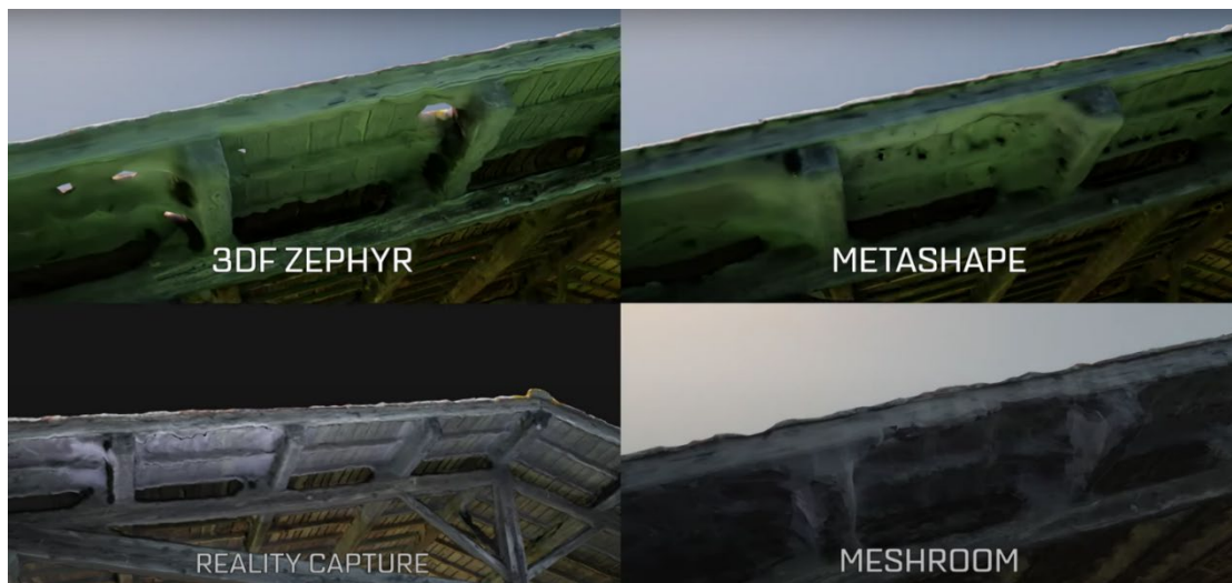
Figure 15 Comparison of the textured mesh reconstructed from cloud points. source: Jérôme Tabeaud, 2023. Which photogrammetry tool is the best?
