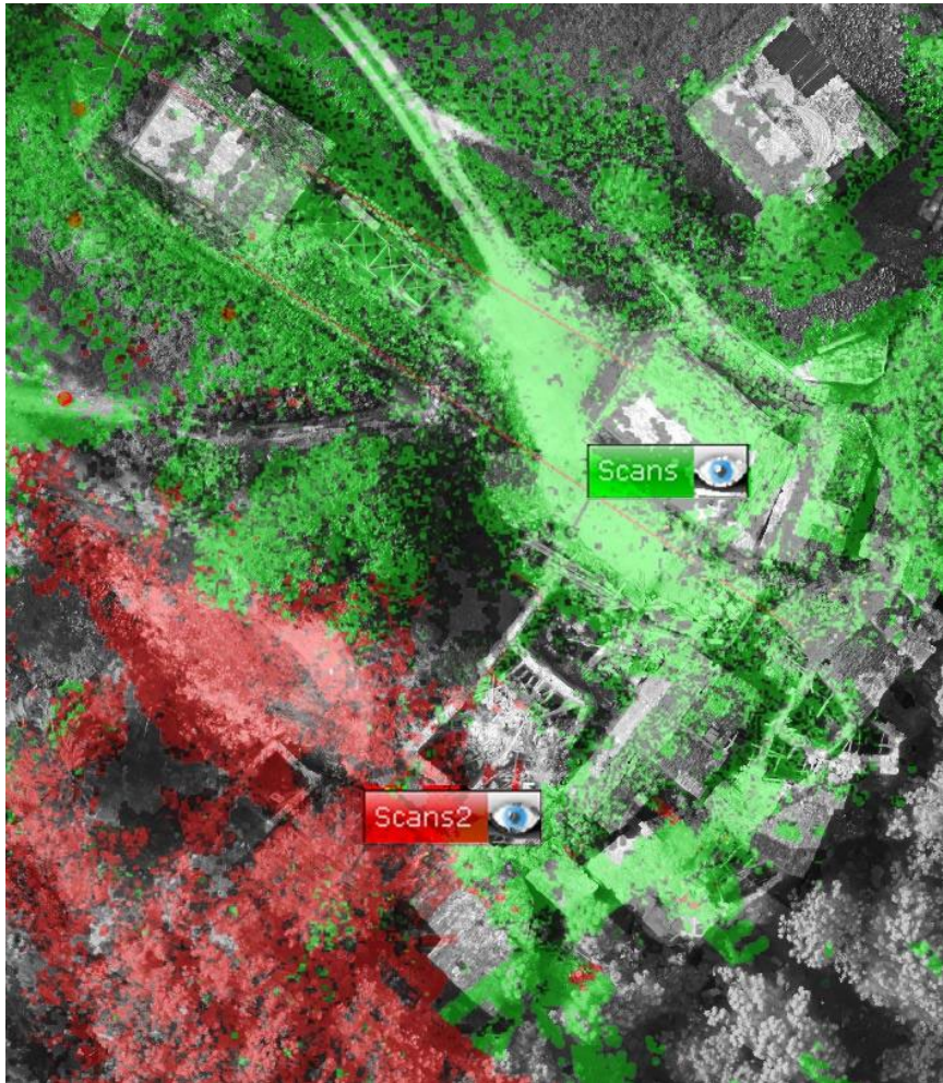
Figure 17: The two groups of scans covering the upper and the lower side of a small village. source: Chiabrando et al 2016
