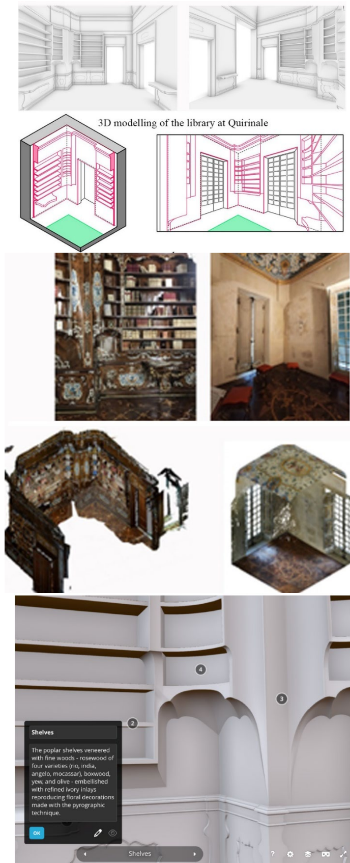
Figure 35 Top right: Rhino 3D model optimized for Virtual visualization. Top left: Photogrammetry and Laser scanning Process. Bottom: The Sketchfab interface allowing to add and edit annotations. Source: Spallone, R., Russo, M., Teolato, C., Vitali, M., Palma, V. and Pupi, E. (2023) 'Reconstructive 3D Modelling and Interactive Visualization for Accessibility of Piffetti's Library in the Villa della Regina Museum (Turin)'
