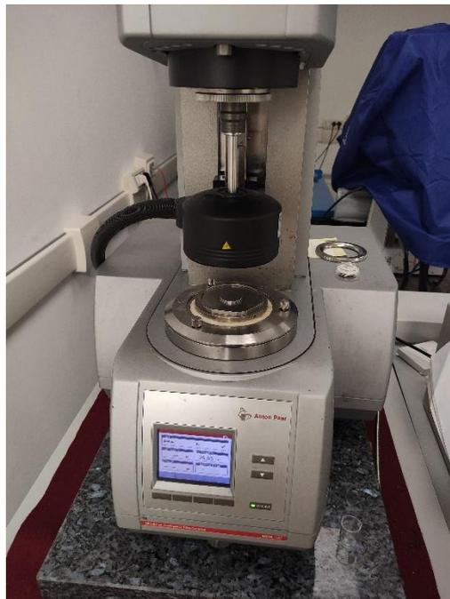
Figura 3.14: Reometro Anton Paar MCR302
