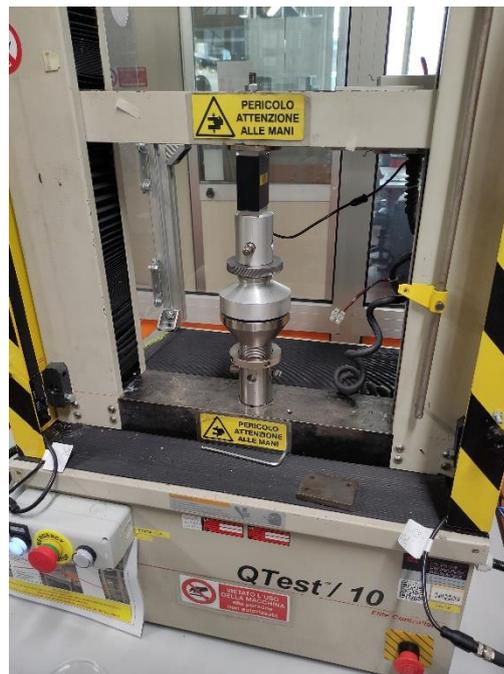
Figura 3.17: MTS QTest™/10 Elite, MTS System Corporation
