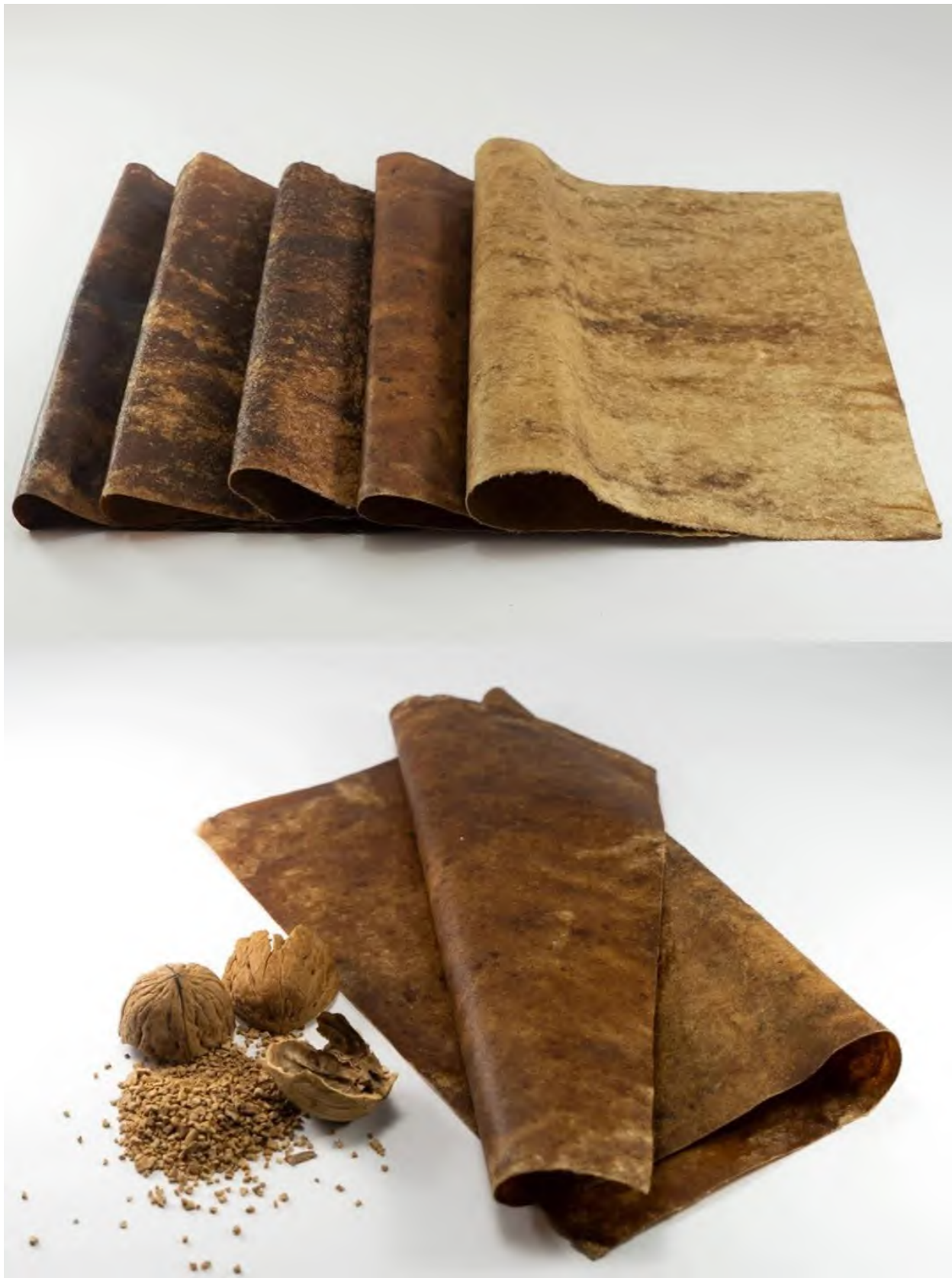
Figure 59 : The leather substitute Kudarat leather synthesized from algae, food and fiber waste
