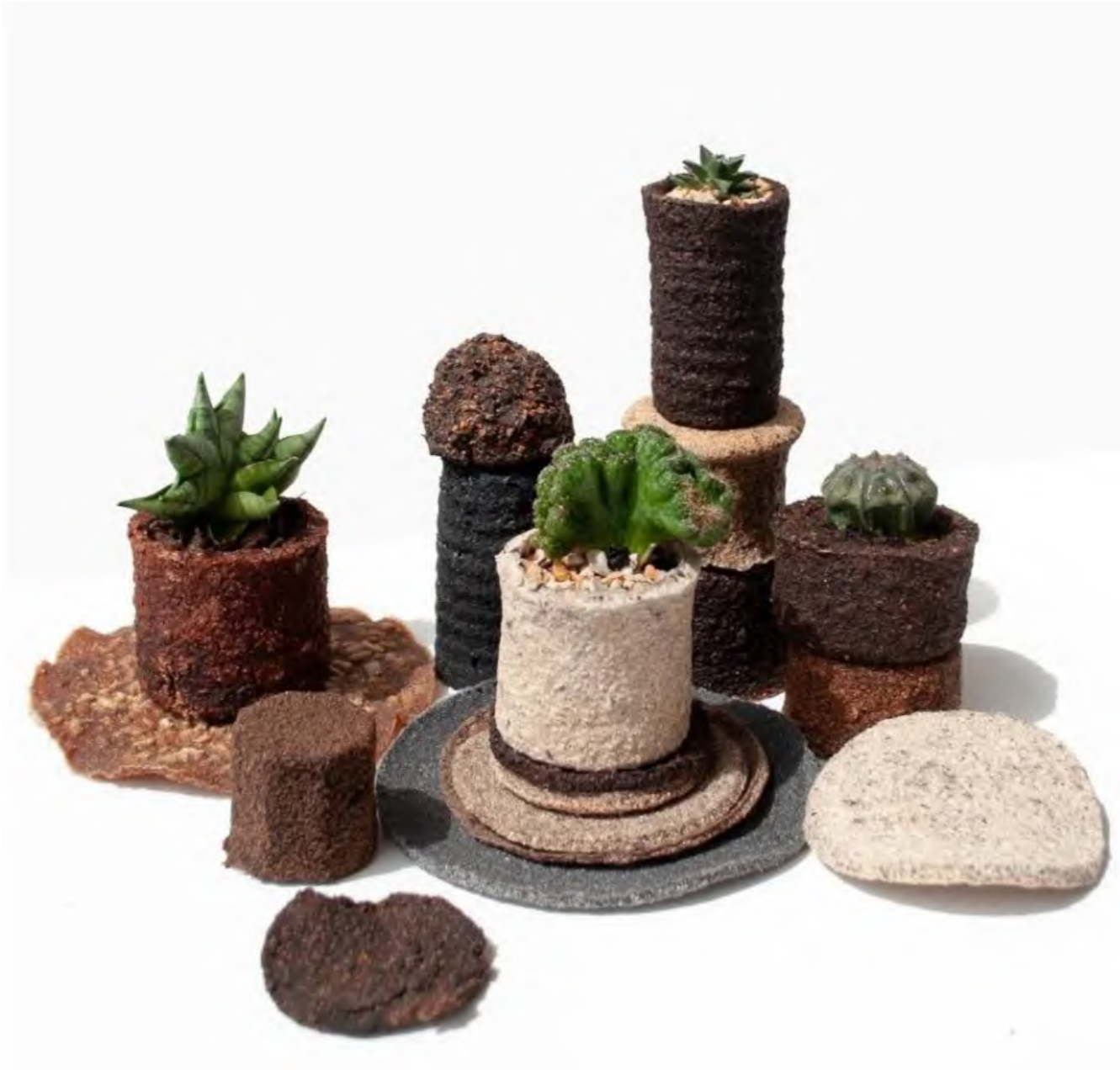
Figure 60 : A flower pot made of agar, glycerin, water and any dried and crushed food waste, designed by Hutsama
