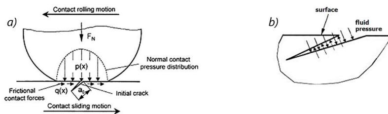
Figure 4: Illustration of surface-initiated crack growth in a moving lubricated contact, showing the distribution of contact forces and the role of fluid pressure in crack propagation.
