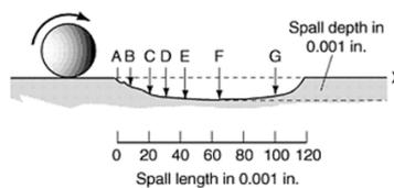
Figure 5: Anatomy of a race spall in a ball bearing.
