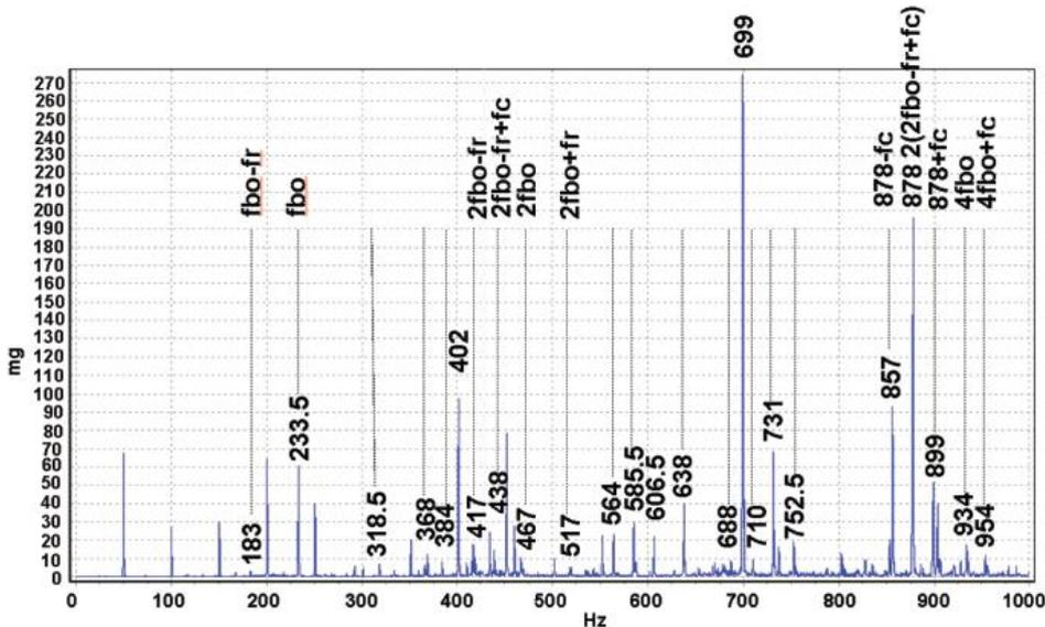
Figure 7. Axial vibration acceleration spectrum on end cap of a 250kW electric motor.
