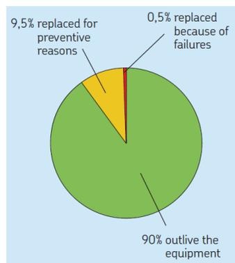
Figure 2: Bearing life and failure estimate from SKF Group.
