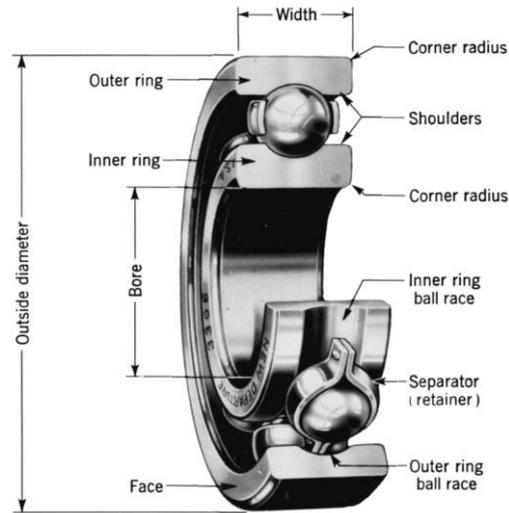
Figure 1: Nomenclature of a ball bearing.
