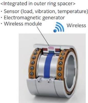
Figure 3: Sensor-integrated bearing unit for machine tool spindles, manufactured by NTN Corporation, equipped with three types of sensors for load, temperature, and vibration measurement. Additionally, the unit includes a built-in generator as an independent power source and a wireless module for wireless data transmission.
