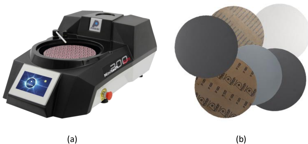
Fig. 41. (a) The Presi machine was used for the grinding and polishing of the samples. (b) The selection of abrasive papers (P480, P600, P800, P1200, and P2400) used for grinding the samples.
