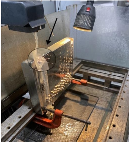
Fig. 35. Illustration of electrical sparks and the movement of water during the wire-cutting procedure.
