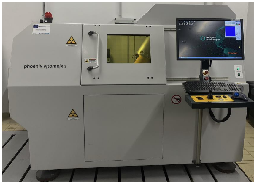
Fig. 39. The software interface checks and alters the sample's position during tomography analysis to keep it in the X-ray imaging frame.
