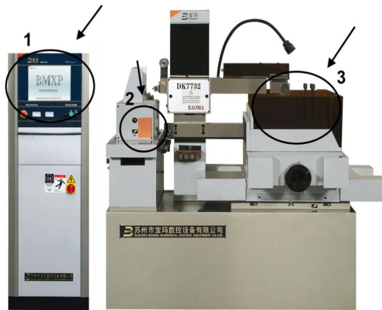
Fig. 34. Key components of the WEDM machine: Section 1 (software controls), Section 2 (coordinate display), and Section 3 (cutting area).
