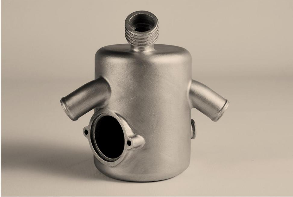
*Figure 8. Engine tank printed with AlSi10Mg [50].*
