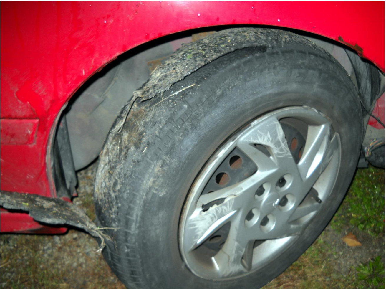
Figura 1: esempi di pneumatico danneggiato e stallamento, "Sunfire Tire Smashed to Bits" by TheDarkThing is licensed under CC BY 2.0 .
