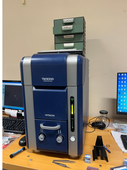
Figure 3.15: Hitachi TM3000 benchtop SEM
