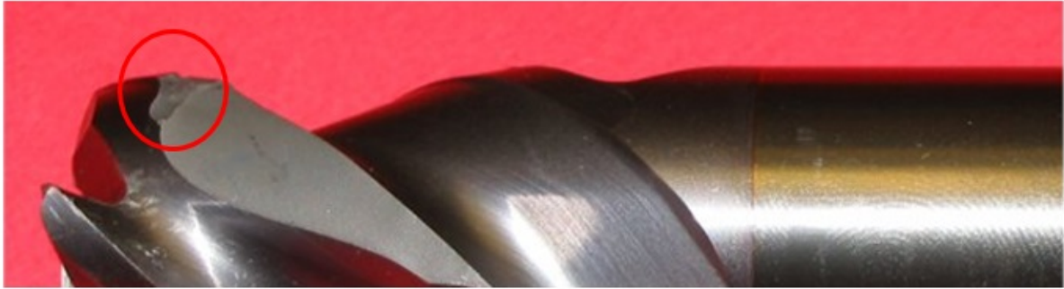
Figure 2.4: Tool Wear Due to Chatter
