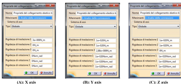
Figure 3.2: Stiffness properties of (A) the rack-and-pinion connection, (B) upper support, and (C) lower support.
