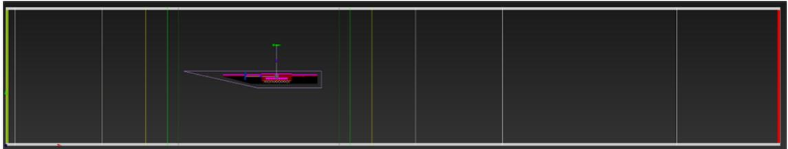
(b) VR Regions stepping away from the test rig. Here it is also possible to notice the domain boundaries, created as thin boxes: the ceiling and floor of the gallery (in white), the inlet (in green) and the outlet (in red).
