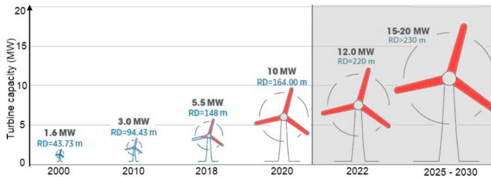
Figure 2.5: Power and rotor diameters of existing and planned offshore wind farms [source: IRENA].
