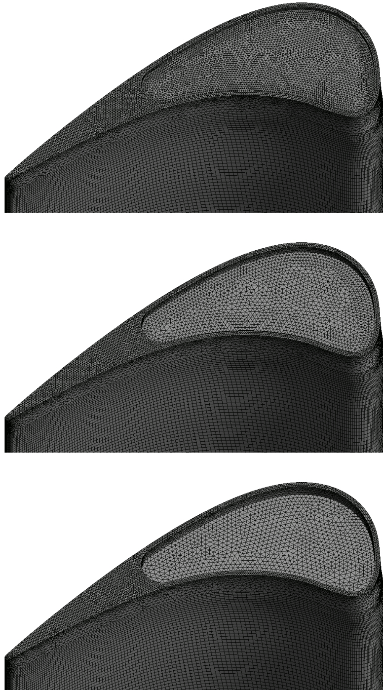
Figure 6.13: Recessed rotor tip with \frac{L_{rec}}{L_{ch}} = 60\% for the three different depths
