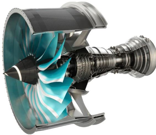
Figure 1.1: Cutaway of an aircraft turbofan engine [1]
