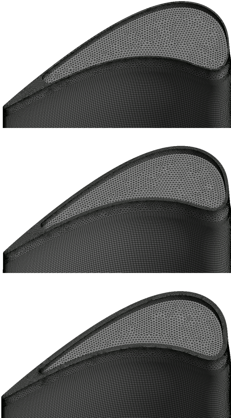
Figure 6.20: Recessed rotor tip with \frac{L_{rec}}{L_{ch}} = 80\% and \frac{h_{rec}}{h_{gap}} = 3 for the three different rim thickness
