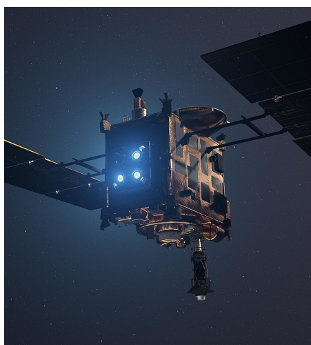
Figure 1.1: Artist's impression of Hayabusa2 firing its ion thrusters. Credits: NASA Science, 2024[ 32]
