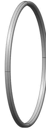
Figure 2.6: CAD view of the lip/unflanged intake
