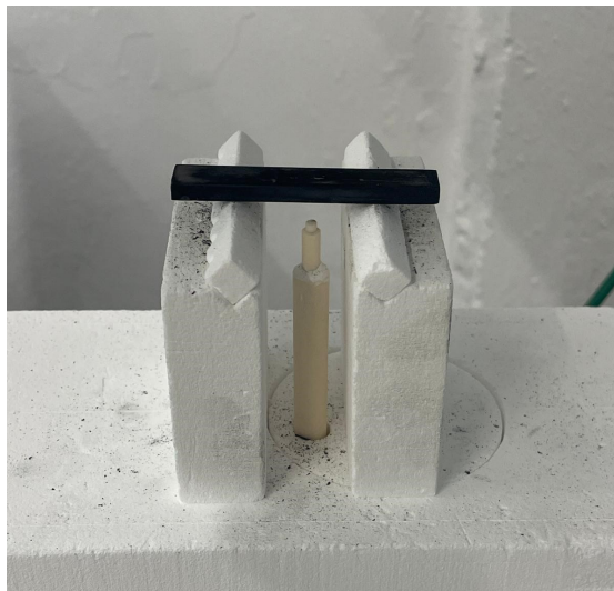
Figure 2.4: Test specimen after the first measurement of elastic modulus in air
