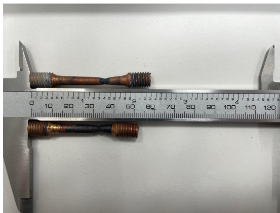
Figure 4.45: Difference in geometry after test at 600°C
