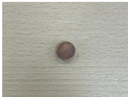
Figure 3.4: CuCrZr specimen used for the CTE measurement
