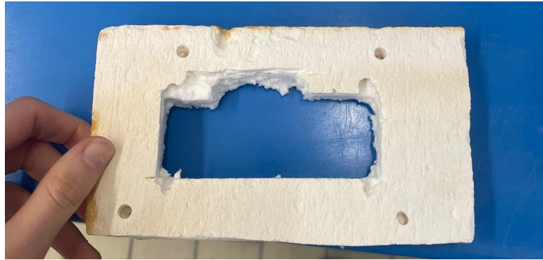
Figure 2.16: Broken structure for measurement of mechanical properties
