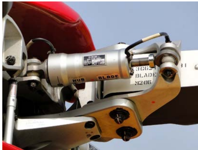
Figure 3: Position of a damper in the rotor
