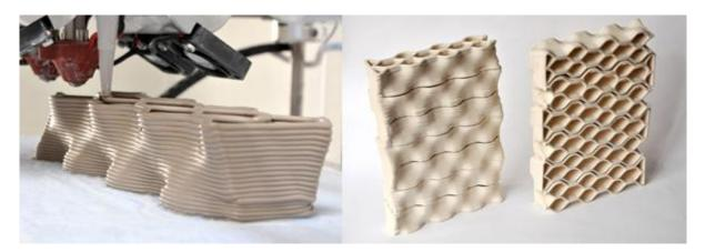
October 2012, B. Peters, *Building Byte*s, in <u>www.deezen.comm</u> Left: 3D molding process of the ceramic brick Right: composition of most ceramic bricks for built a wall or a shading system
